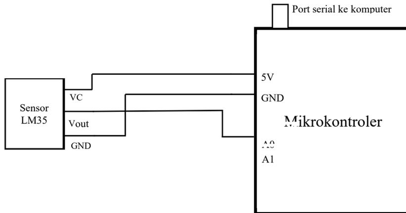
Figure 2. Circuit temperature sensor system
