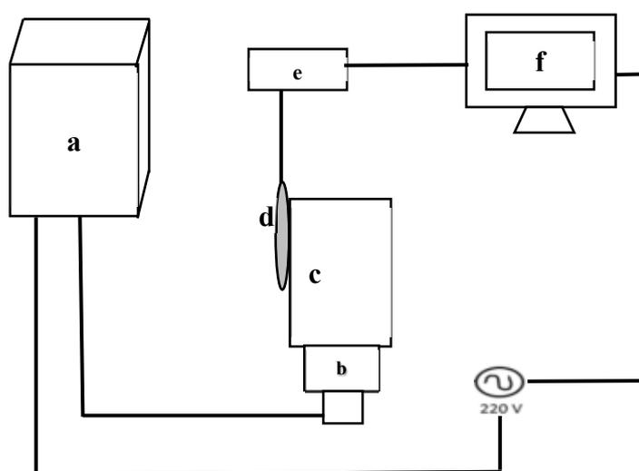
Figure 1. UAE System Design. a: ultrasonic generator, b: transducer, c: reactor tube, d: temperature sensor, e: microcontrpler, f: computer.
