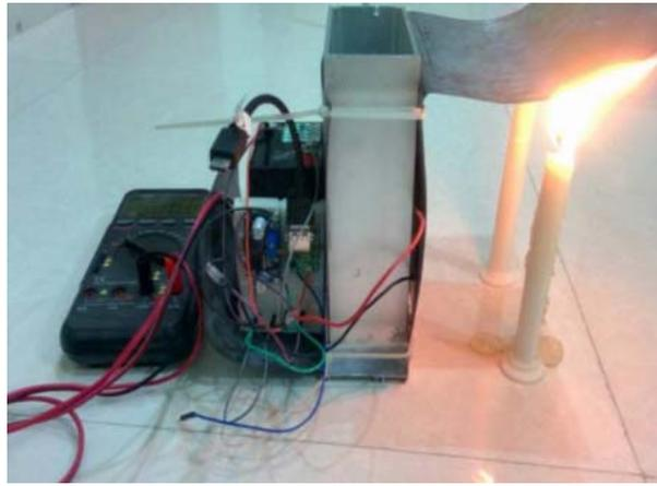
Fig. VI: Experimental setup for the thermoelectric generator in related work
