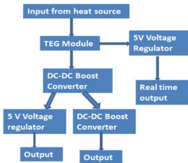
Fig.V: Thermoelectric generator block diagram for related work
