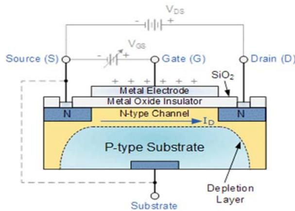
Fig. IV: Structure of the MOSFET (power transistor) [9]
