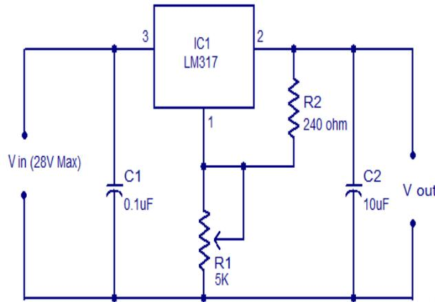
Fig. VIII: 0 to 25 volts regulator circuit [8]
