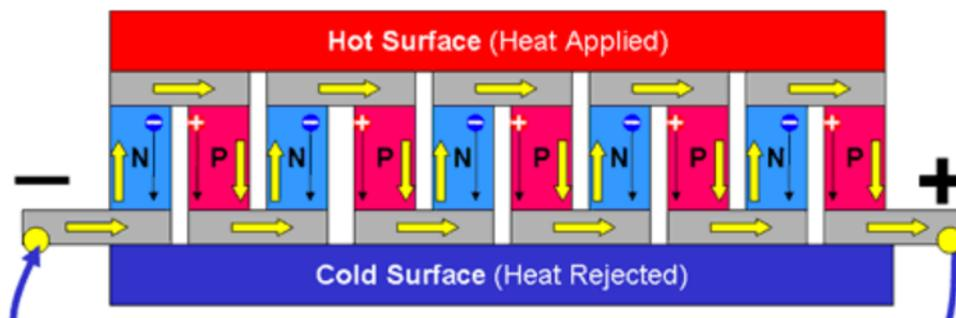
Fig. II: working principle of a thermoelectric generator
