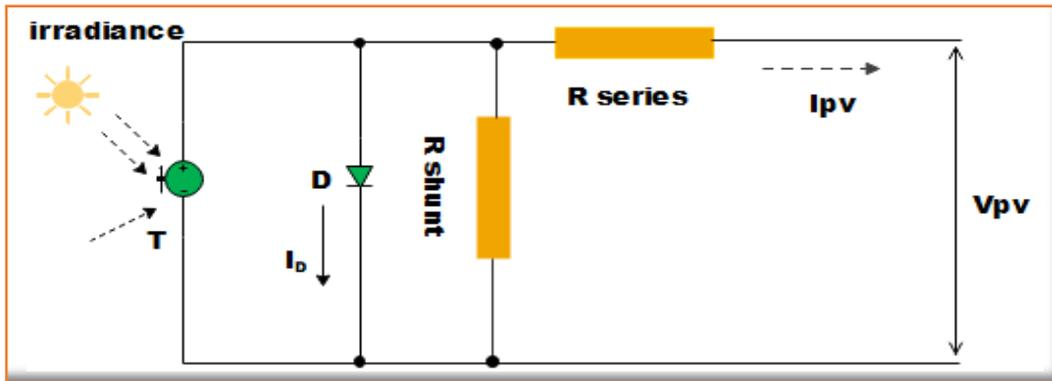
Fig.2. Sight model of a tandem photovoltaic cell.
