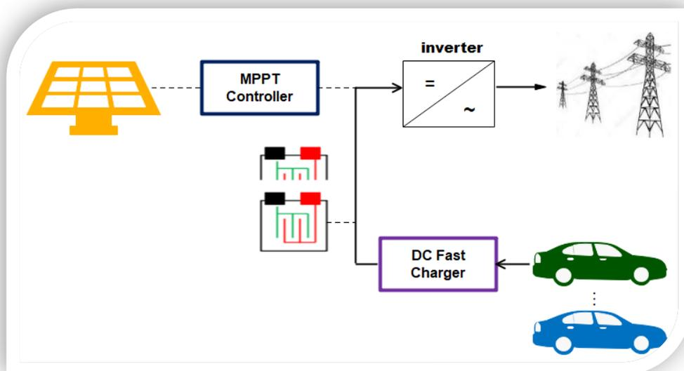
Fig.1. A fleet of electric vehicles to charge a grid.
