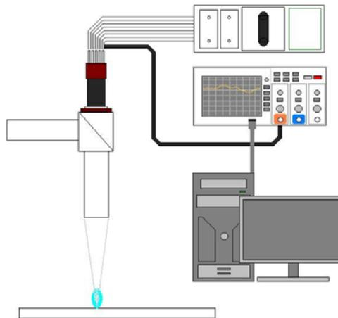
Fig.4. – The general scheme of the experiment on testing the mock-up monitoring system based on the "FEU-35" photomultiplier tube.
