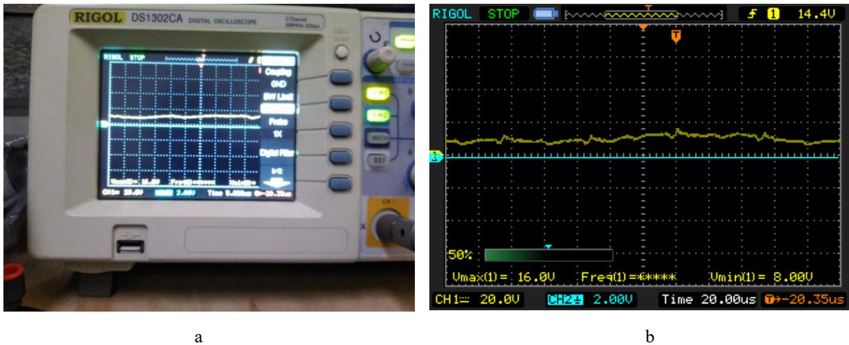
Fig.3. – a - “RIGOL” digital oscilloscope used in testing the layout of the mock-up monitoring system based on the "FEU-35" photomultiplier tube. Fig.3b shows the analogue signal on the oscilloscope screen as well as the already processed signal.
